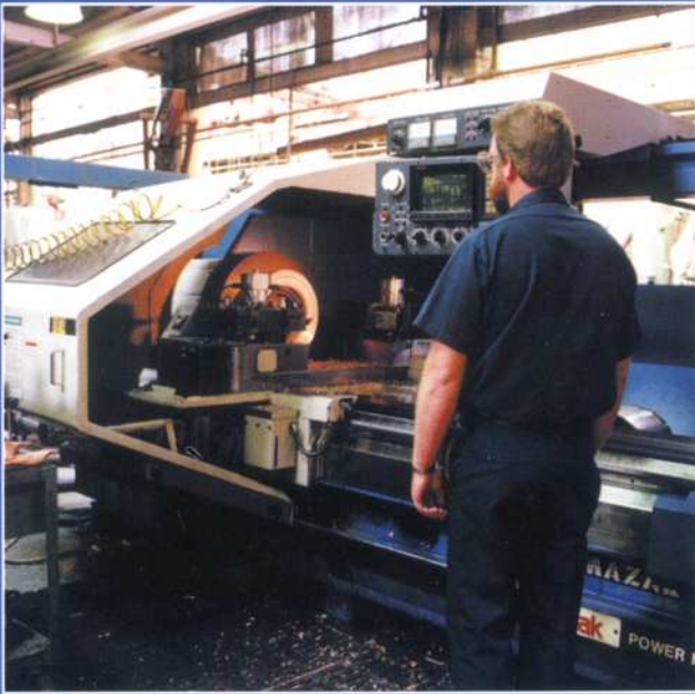
Rings are machined to precise tolerances and premium quality surface finish.
